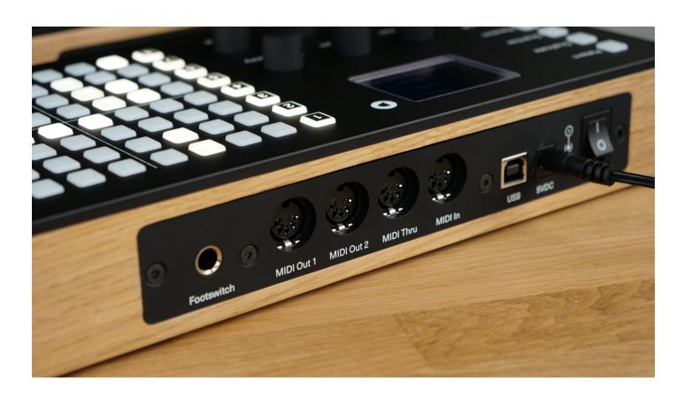
The Seq is equipped with a wide array of inputs and outputs. This allows communication with a wide variety of devices. The Seq also allows feeding tracks with MIDI notes using MIDI controllers. While looking at the
