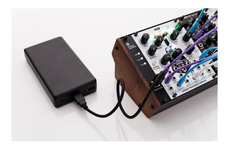
Recommended minimum power bank efficiency is 2.4A/5V. Check the needs of the rig using Polyend Anywhere power bank amperage requirements chart.
