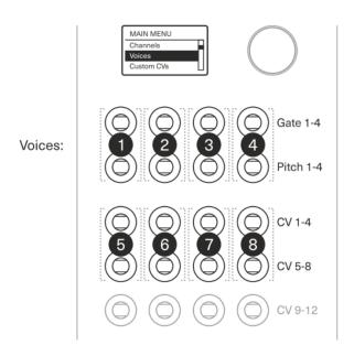
The number of occupied voices determines the remaining configurable outputs. The system allows you to configure only the non-occupied outputs. For example, if voices are set to 7, then configurable CVs are CV4, CV8, and CVs from 9-12.
