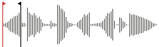
Fade In applied at the start of the audio to create a smooth volume transition to begin.
