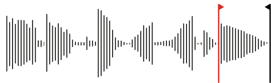
Fade Out applied at the end of the audio to create a smooth volume transition to conclude.
